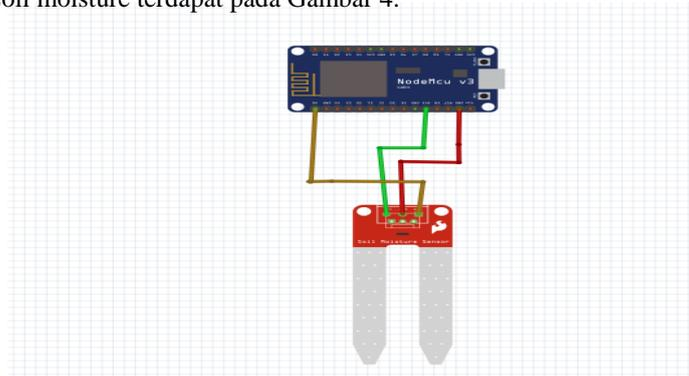
**Gambar 4.** Rancangan Sensor Soil Moisture
