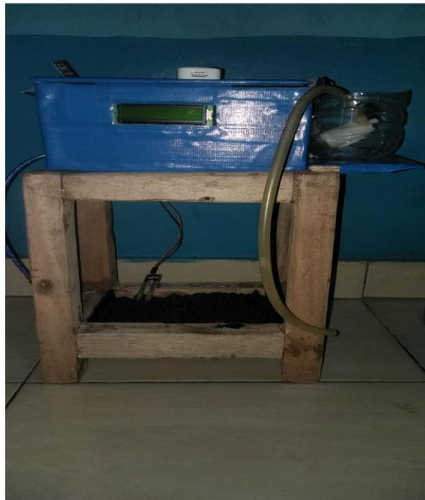
**Gambar 8.** Sistem Monitoring Suhu Dan Kelembapan Tanah
