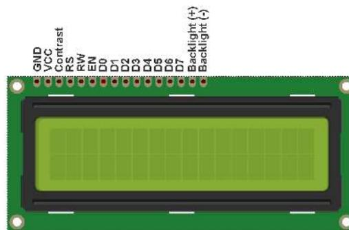
**Gambar 4.** LCD (*Liquid Crystal Display*) 16x2
